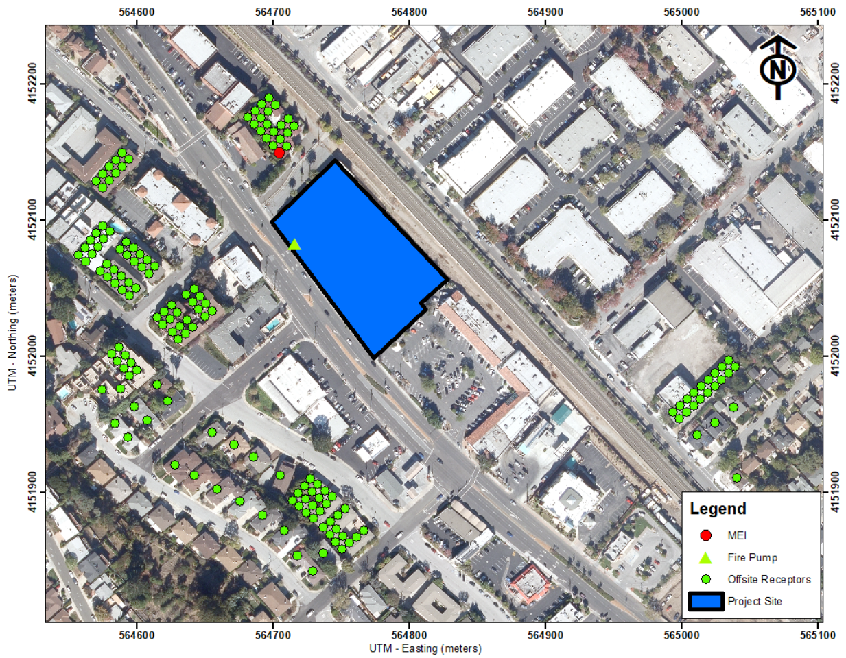
Figure 1. Locations of Project Construction Site, Fire Pump, Off-Site Sensitive Receptors, and Maximum TAC Impact Location (MEI)
